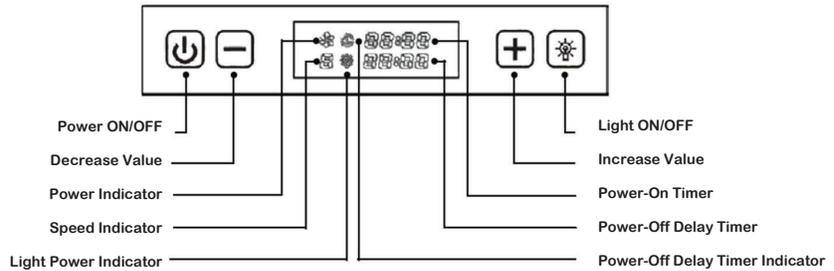
**Power:** Power ON/OFF the range hood and activate power-off delay timer.
